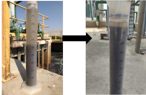
Figure 3: Before and After the dewatering Process for case A
